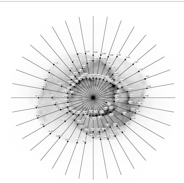
**Figure 10:**  $\omega$  and Radial Intensity Profiles The resulting  $\omega$ 's from careful fitting of radial profiles along the lines shown in the figure.  $\omega$  is measured in milliarcseconds/ year (from Reed et al., 1999).
